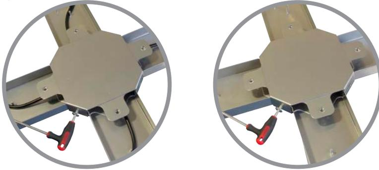
Carefully position and lower octagonal centre cover onto bottom support plate. Align two side holes of cover to any thread fixings of bottom support plate. Insert and tighten two hex socket screws to secure octagonal centre cover.
