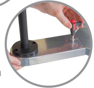
Depress all lock buttons on underside of bottom support plate and insert and tighten remaining four hex socket screws to secure plates. Please gently lift end of bottom support plate, if required, to allow hole in top support plate to align to thread fixing in octagonal centre cover.
