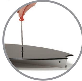
Pre-assemble the two black acrylic shelves to 616mm profiles by aligning the predrilled holes, inserting 4 off countersunk self-tapping screws, and tightening with cross-head screwdriver supplied to secure.
