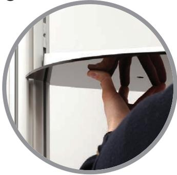
Ensuring the black acrylic is lowermost, slide and raise second assembly into the same post channels as the previous enclosure until the expanding clamps come into contact with the bottom of the pre-installed locator bars of the upper posts. Tighten grub screws in ends of profile to secure in position.
