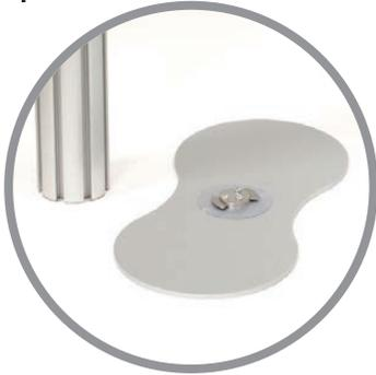
Place base plates on the floor, position posts (with single bracket) centrally over male fitting of base plate (A), and rotate until assembly drops into position, continue rotating clockwise through 90° to secure (B).
